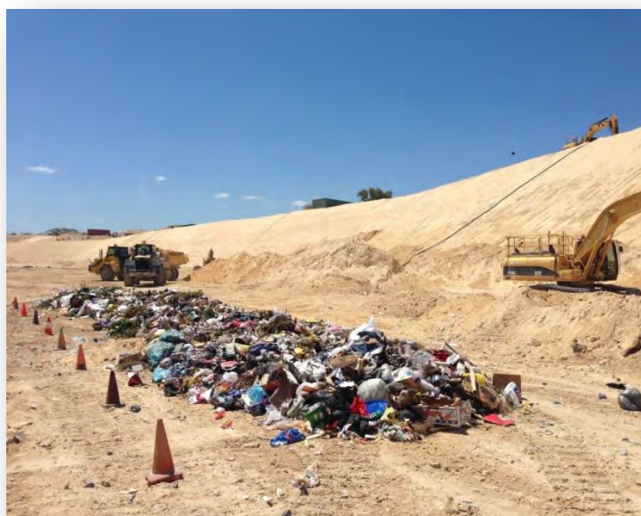
Victoria Park load prior to audit. Orange witches hats spaced 3m apart, load width is 4.5m. Auditors walked on both sides along length of waste and recorded observations
