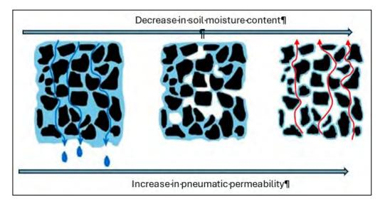
**In the diagram above** (not to scale and illustrative only) the blue lines represent the direction of travel of irrigated leachate/rainwater down through and into the temporary capping and top layers of waste in the landfill. By filling the gaps in the granular structure of these layers, greater resistance is provided against landfill gas rising through the landfill to the surface. In
